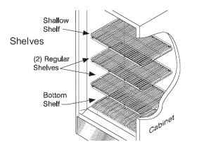
The appliance is provided with 4 shelves. One goes the floor of the cabinet and the other 3 are placed in the metal side supports wherever they are needed. shallow shelf goes in the upper position.
