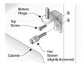
6. Slide bottom hinge onto hex spacer and attach top screw to cabinet . Retighten both hex spacers.
